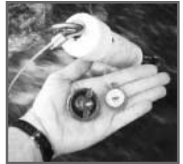
Cook Inlet Keeper has increased sampling frequency in salmon streams by deploying temperature loggers (StowAway TidbiT3™ by Onset) which collect data at 15-minute intervals.
