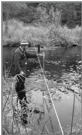
Ole Andersson of the Kenai Watershed Forum measures discharge on the lower Ninilchik River.
