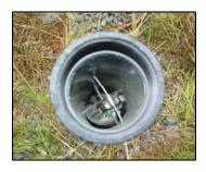
Glue the female adapters to each end of the PVC pipe. Drill a hole for one eyebolt to go through a clean out plug. Drill at least 20 holes in PVC to allow water flow. Secure the eye bolt through the clean out plug with appropriate-sized nuts and bolt. Use a cable tie through drilled holes to suspend the data logger in the housing. Additional cable ties can be used to secure rocks in the bottom of the housing to weigh it down. Screw the clean out plugs into the female adapters.
