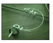
Materials: 1/2" rebar (4' length) 3/8 " x 4" ZC eye bolt (1) 9/16 - 1 1/16 hose clamp (3) 1/8" wire rope clip (2) 1/8" RL uncoated cable (2' length)
