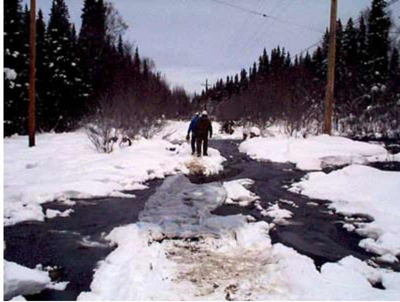
Figure 2. January 7, 1999 photo of the Unocal 6” gathering pipeline spill in the Kenai National Wildlife Refuge. Black liquid is the released pipeline contents, which melted the three feet of snow present. Photo source: Alaska Department of Environmental Conservation website.
