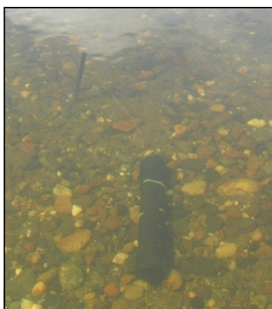
Water data logger is inside PVC housing and secured by cable to rebar.
