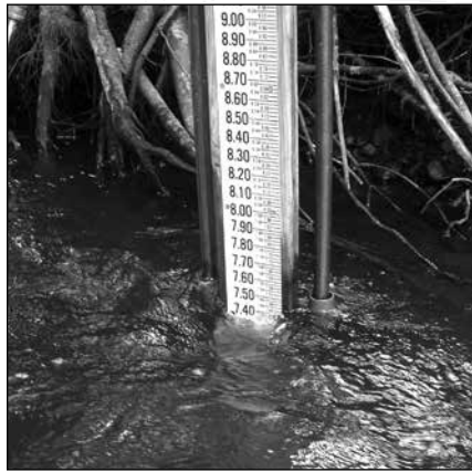
The new camera-based system will focus on an instream ruler (or staff plate) and capture stream level data to track changing water availability in salmon habitats.
